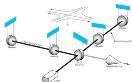
Above and following page: Diagram and photos of the LIGO Hanford Observatory in Hanford, Wash. (Courtesy of LIGO Laboratory)
