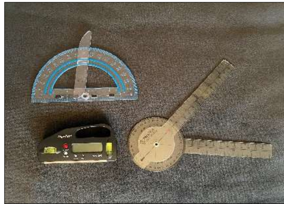
FIGURE 6. Protractor with Swing Arm (top left), Electronic Angle Gauge (lower left), and Medical Goniometer (right).
