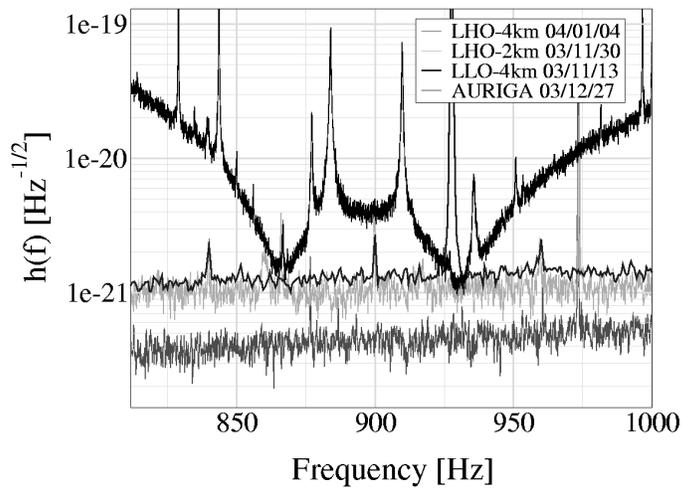
**Figure 2.** Best single-sided sensitivity spectra of AURIGA and the three LIGO interferometers during the joint observation. In the AURIGA spectrum, several spurious lines are visible while LIGO spectra present calibration lines at 973 Hz for the Hanford detectors (LHO-4 km and LHO-2 km) and 927 Hz for the Livingston detector (LLO-4 km).
