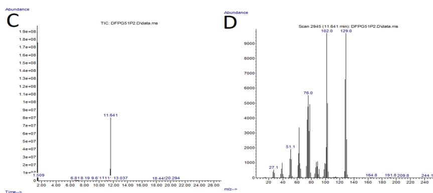
Figure C and E represents analysis for phase 2 for synthesizing the isooxazoline core motif. Figure D shows the mass spectroscopy data of the core motif breakdown at 11.641 minutes as seen on figure C. There are peaks at 129.0 m/z, 102.0 m/z, and 76.0 m/z that represents different parts of the molecule when being broken down.
