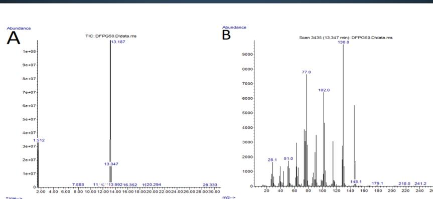
Figure A is the chromatogram of phase 1 in representative of the molecule of interest, cinnamaldehyde oxime, with the breakdown of the molecule on figure B. Figure B represents the shows multiple peaks at that 13.187 minutes, Figure A. There is a peak at 148.1 m/z and two large peaks at 130.0 m/z and 77.0 m/z.
