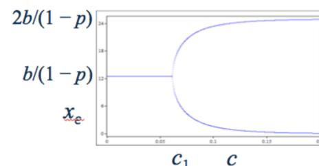
Figure 2: Bifurcation diagram showing steady states of system as a function of crowding factor  $c$
