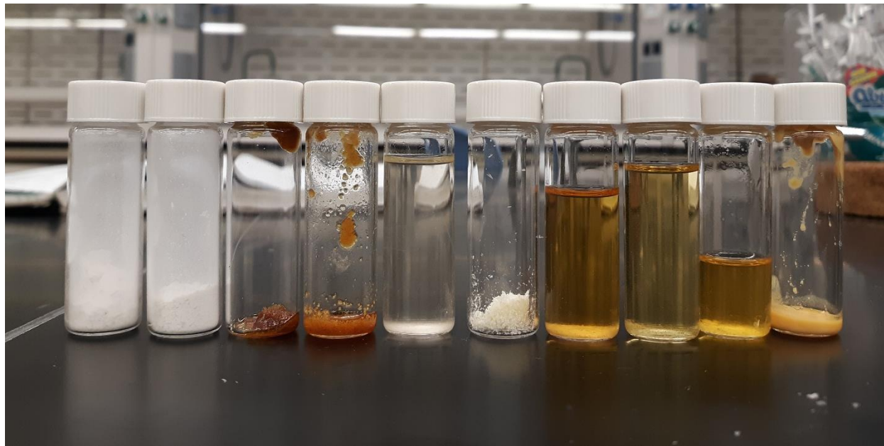
Figure 3. Products Obtained from the Ten Trials (labeled #1-10 from left to right). Products #5, #7, #8, and #9 have been dissolved in ethanol to easily transfer the product from the round bottom flask after using the rotary evaporator to the vial to store the product.
