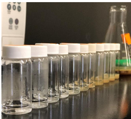
Figure 1: AgNPs produced using Ag 2 O and citrate through microwave heating. This describes the color transition of AgNPs as heat time increases.
