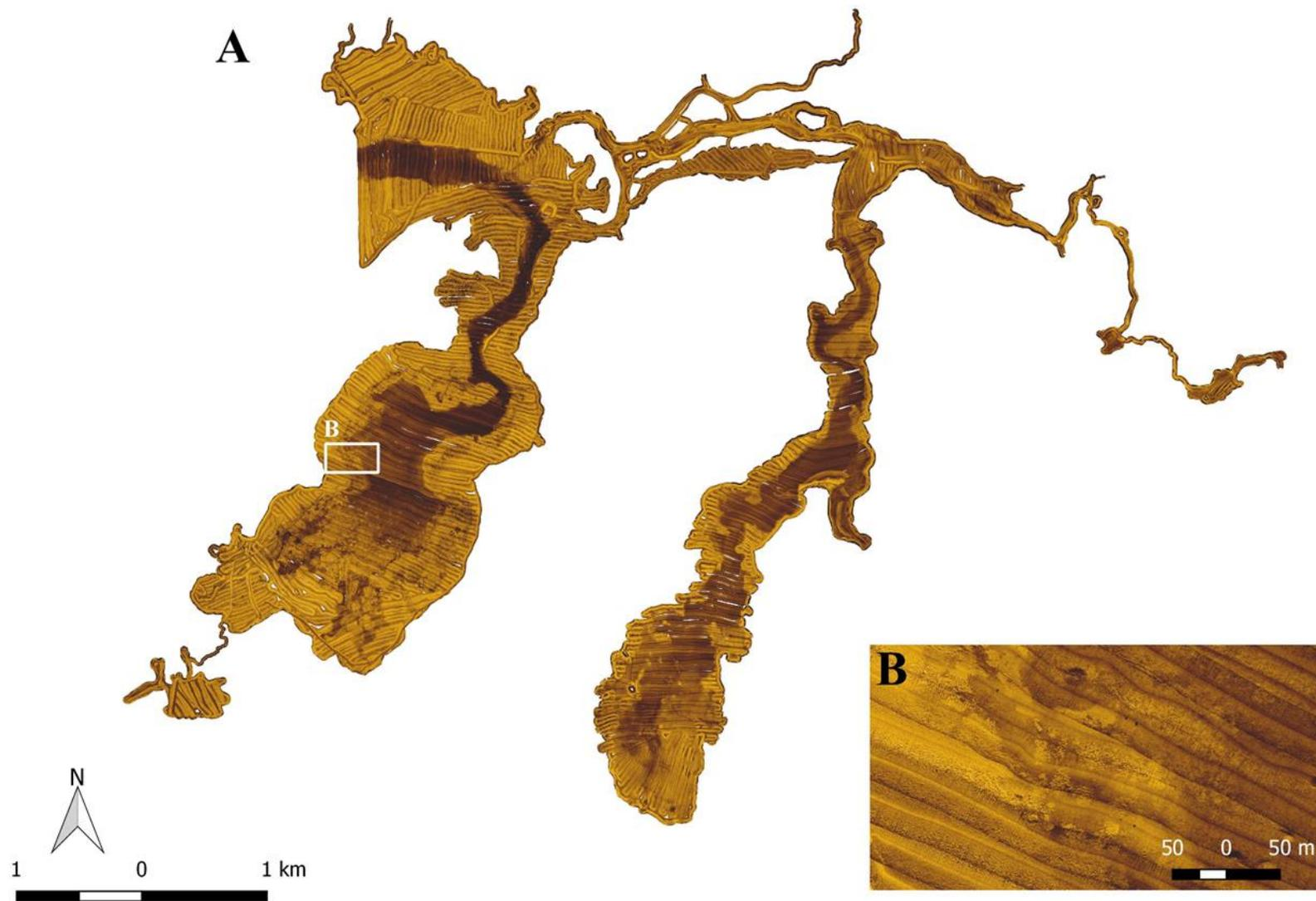
Figure 7. A) Sonar mosaic of the San Pedro lagoon system. B) Close-up of sonar tracks.
