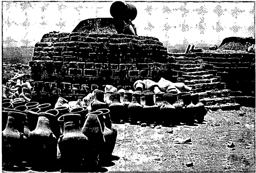
Fig. 22.8. The two round kilns, connected by steps, have open roof tops through which the pottery enters the kilns. On the crown of each kiln stands a temporary dome-shaped mud construction which is dismantled to remove the fired wares. The fire boxes are behind each kiln.
