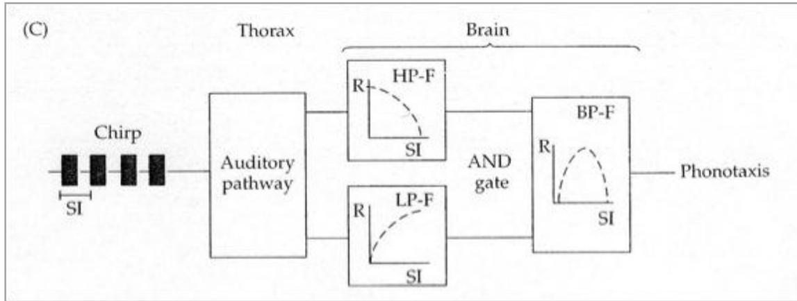
**Figure 2.** Diagram of the Schildberger model showing the high-pass filter (HP-F) and the low-pass filter (LP-F) combining to form a band-pass filter (BP-F), used to explain the optimal phonotactic response to mid-range syllable periods (modified from Carew, 2000).
