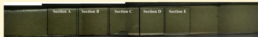
Figure 4. A low magnification of the sample showing the small tear. Sample is cut into small pieces for SEM imaging.
