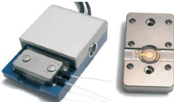
**Figure 2.** Product images of QCM-D sensing chamber and crystal
